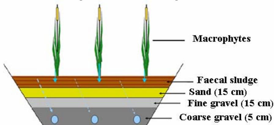
Figure 1: Diagram of a planted drying bed
