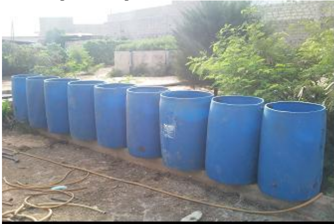
Photo 1 : Experimental scale drying beds
