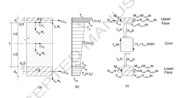
Fig. 1: Geometry, temperature and stress resultants: (a) Geometry (model I and II); (b) Temperature Distribution; (c) Stress resultants (model I).
