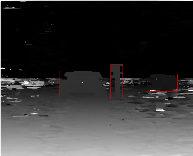
Fig. 14. Disparity map of the stereo pair of the figure 7 with bounding boxes
