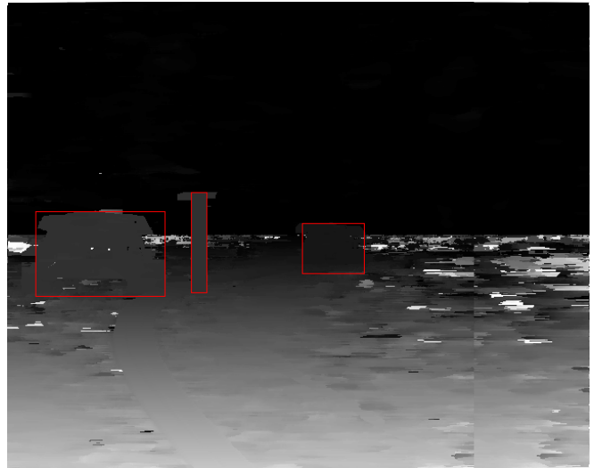
Fig. 15. Disparity map of the stereo pair of the figure 8 with bounding boxes
