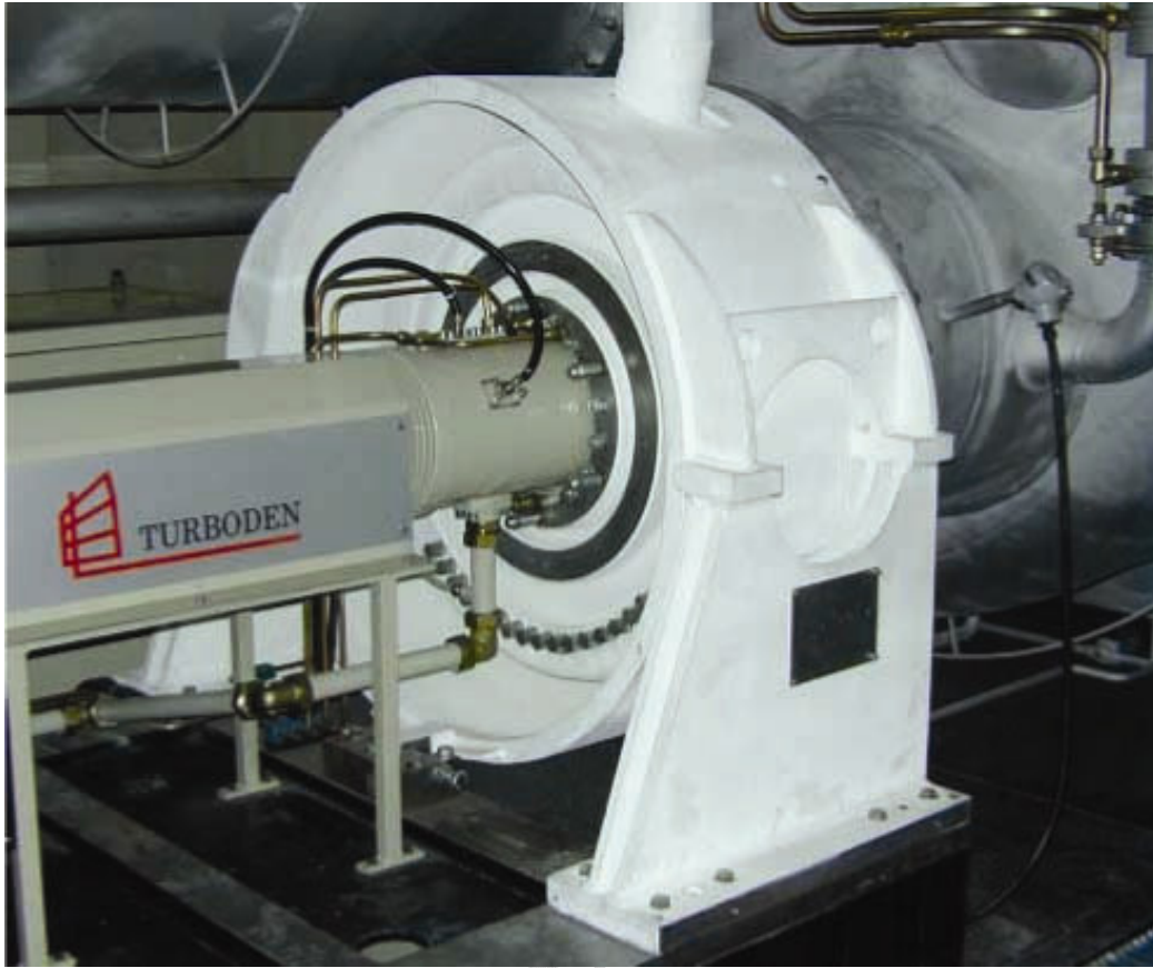
Fig. 10 Two-Stage Axial Turbine for the Biomass-Fired ORC Process (from Ref. 25)
