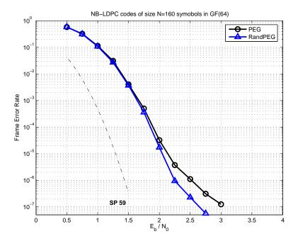
Fig. 1. Performance comparison for the design of non-binary LDPC codes: two codes whose underlying Tanner graphs were constructed with respectively the PEG and RandPEG algorithm are simulated over a BIAWGNC. The sphere packing bound of 1959 (SP59) [9] gives a lower bound on the block error probability for this codeword length.
