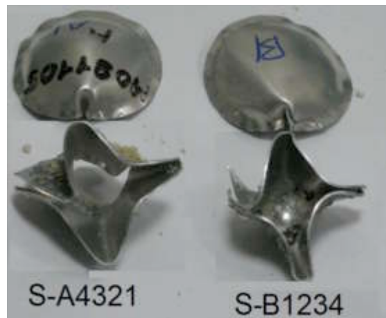
Figure 10 Post mortem photos sandwiches under quasi-static perforation
