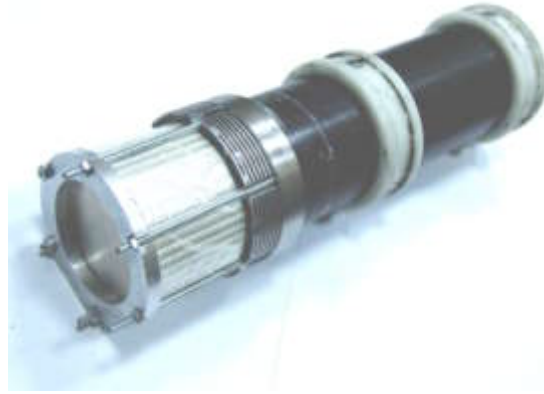
Figure 4. Photograph of the projectile/specimen system
