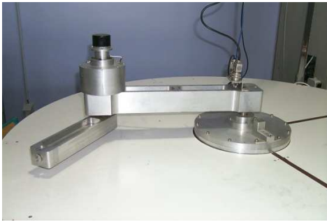
Fig. 8. The scara robot prototype.
