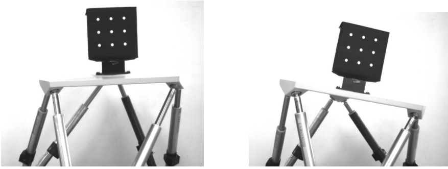
Fig. 5 Initial (left) and desired (right) position of the end-effector, seen from the camera.
