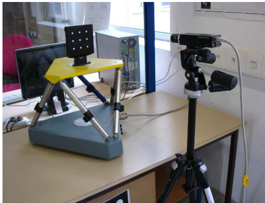
Fig. 1 A Gough-Stewart platform observed by a camera.
