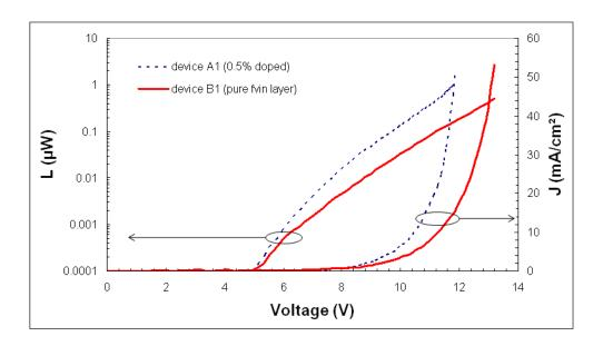
fig 5 : J-V and L-V curves for a low-doped (0.5% of FVIN in  $Alq_3$ , device A1) and a pure (20 nm neat film, device B1) EML.
