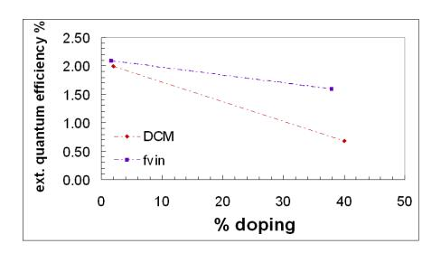
fig 9 : Comparison of external quantum efficiency in  $FVIN:Alq_3$  and  $DCM:Alq_3$  OLEDs at low and high doping level.
