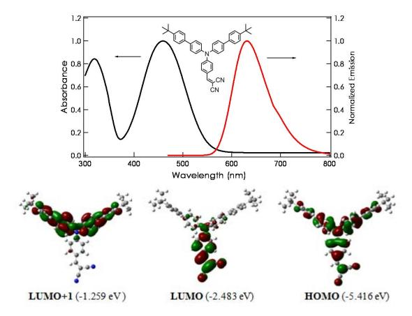
Fig 1: (a) (from [9]) Normalized absorption and emission spectra of FVIN in thin films (inset: FVIN chemical structure). (b) TDDFT computations (B3LYP, 6-31G(d)) of FVIN in the gas phase. Representation of the electronic density of the HOMO, LUMO and LUMO+1.
