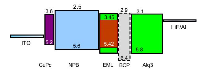
fig 2 : OLED architecture used in the experiments together with HOMO-LUMO levels in eV. For FVIN (EML), the LUMO level is deduced from the HOMO and the optical gap. The other levels are taken from the literature.
