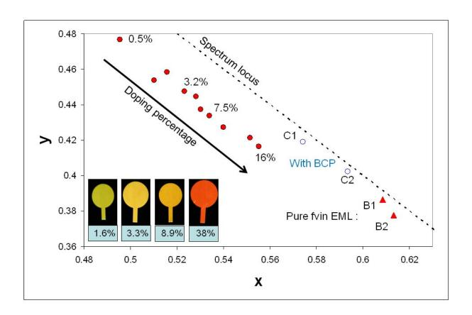
Fig 6: Evolution of the CIE (x,y) coordinates with the doping level for devices A, B and C. The dots are the doped devices (filled ones without BCP (A), empty ones with BCP (C)) whereas the triangles are the pure-EML devices (B). Inset: photos of four OLEDs with different doping level (color online).
