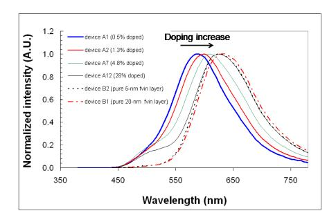
fig 3 : evolution of the fluorescence OLED emission spectra in A and B configurations for different doping levels of FVIN in Alq<sub>3</sub>.
