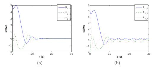
Fig. 1. Trajectories of the triple integrator system under feedback (10) (a) without perturbation (b) with perturbations.
