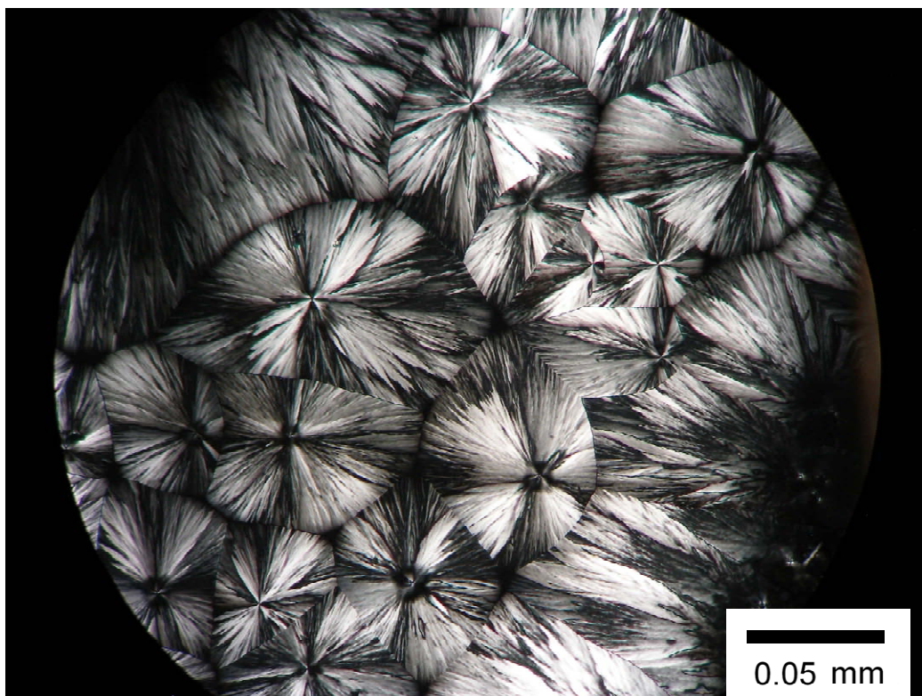
Figure 8. Polarized optical micrograph showing spherulites resulting from PEG crystallization.
