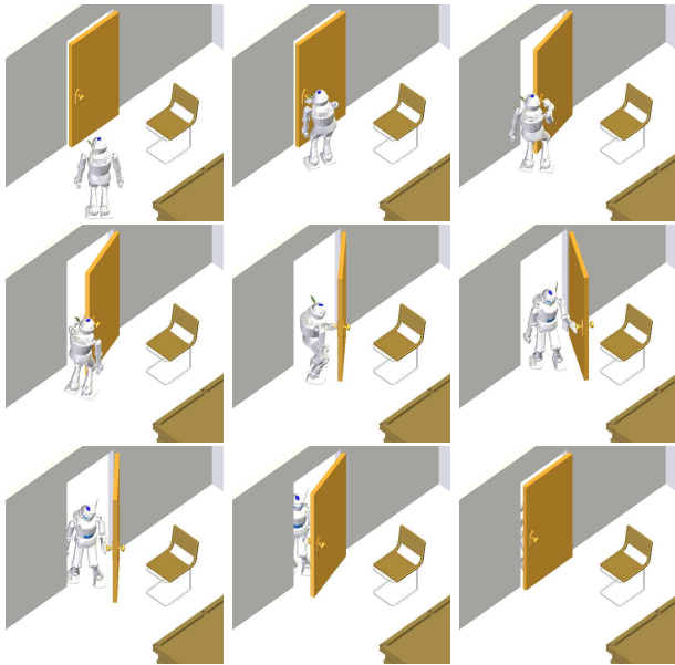
Fig. 6. Opening and closing a door with two hands. A chair stands in the way of the door, so the robot has to go through a narrow passage between the door and the wall.
