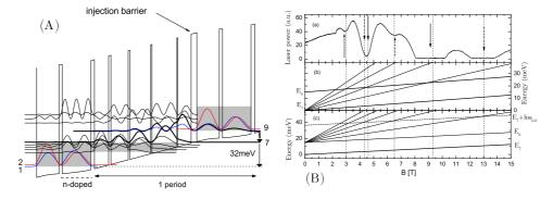
Fig. 1. (A) Self-consistent solution of coupled Schrodinger and Poisson's equations for one period of the structure. Layer sequence is given in Ref. 8. (B) (a) Emitted power as a function of the magnetic field under a constant current  $J = 236 \text{ A.cm}^{-2}$ . (b) and (c) Fan charts of the laser LLs. Note in (b) the crossing at 9, 4.5 and 3 T; and in (c) the crossing at 13, 6.5 and 4.3 T.
