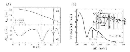
Fig. 3. (A) (a) Dark current as a function of B. (b) Same curve where the continuous contribution has been subtracted. (B) Fourier Transform amplitude of experimental  $\Delta I_{dark}$  vs  $\Delta E$  (see text).
