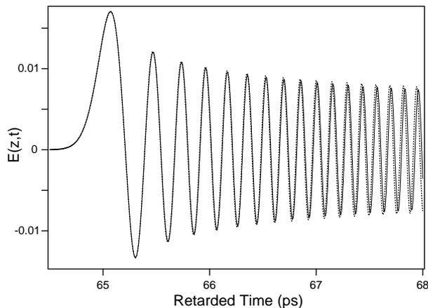
Figure 1: Brillouin precursor obtained for the parameters of the figure 3 of [1], that is for  $\omega_0 = 3.9 \times 10^{14}$  rad/s,  $\omega_c = 3.0 \times 10^{14}$  rad/s,  $\omega_p = 3.05 \times 10^{14}$  rad/s,  $\delta = 3.02 \times 10^{10}$  rad/s, and  $z = 7.232 \times 10^{-2}$  m. The full line is the exact numerical solution obtained by fast Fourier transform (FFT) and the dashed line is the approximate analytical solution given by Eq.7.
