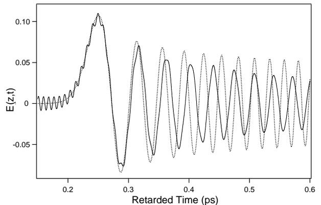
Figure 2: Same as Fig.1 for the parameters of the figure 5 of [1], that is for  $\omega_0 = 3.9 \times 10^{14}$  rad/s,  $\omega_c = 3.0 \times 10^{14}$  rad/s,  $\omega_p = 3.05 \times 10^{12}$  rad/s,  $\delta = 3.02 \times 10^{12}$  rad/s, and  $z = 2.290$  m. The rapid oscillations of small amplitude superposed upon the beginning of the Brillouin precursor are the end of the Sommerfeld precursor.
