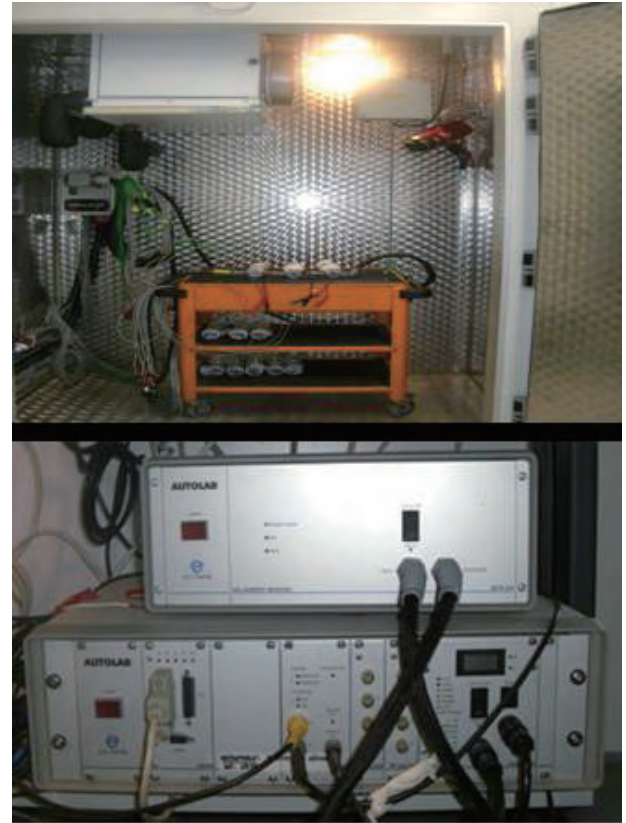
Figure 2: The climatic chamber and used measurement devices of battery impedance
