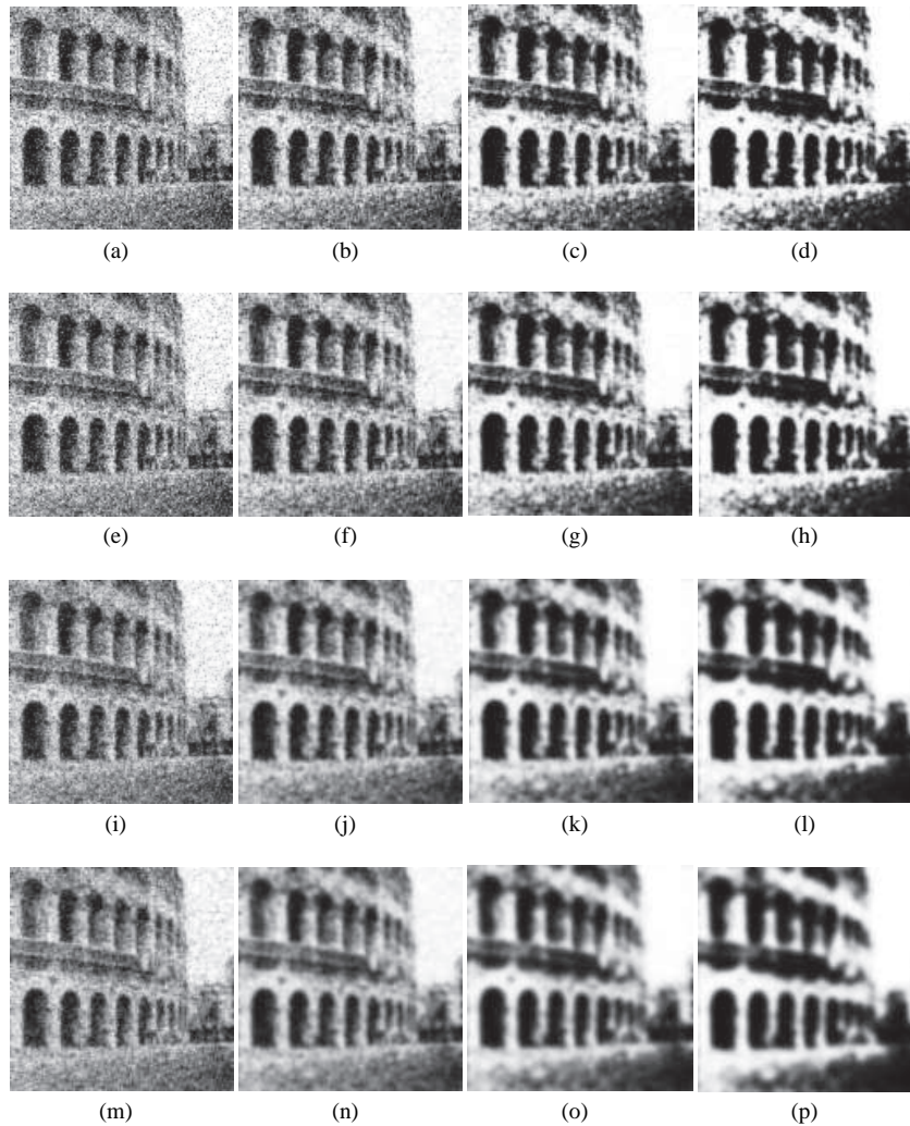
FIGURE 30. : Noise filtering of the image represented in Fig. 29. (a), (b), (c), (d). Filtered image obtained for D = 0.075 and for the respective processing times t = 1 , t = 3 , t = 6 and t = 9 . (e), (f), (g), (h) Filtered image obtained for D = 0.1 and for the respective processing times t = 1 , t = 3 , t = 6 and t = 9 . (i), (j), (k), (l) Filtered image obtained for D = 0.2 and for the respective processing times t = 1 , t = 3 , t = 6 and t = 9 . (m), (n), (o), (p) Filtered image obtained for D = 0.3 and for the respective processing times t = 1 , t = 3 , t = 6 and t = 9 .
