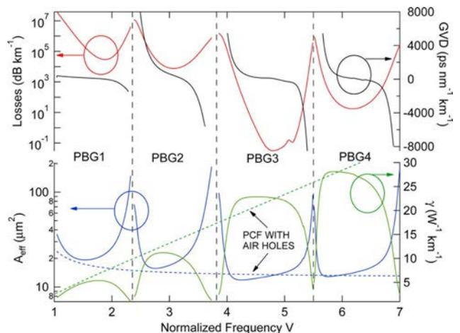
Fig. 1. (Color online) Top axes: loss (red, left) and GVD (black, right) as a function of normalized frequency  $V$ . Bottom axes: effective area  $A_{\text{eff}}$  (blue, left) and nonlinear parameter  $\gamma$  (green, right). The dashed curves show results for an index-guiding PCF.
