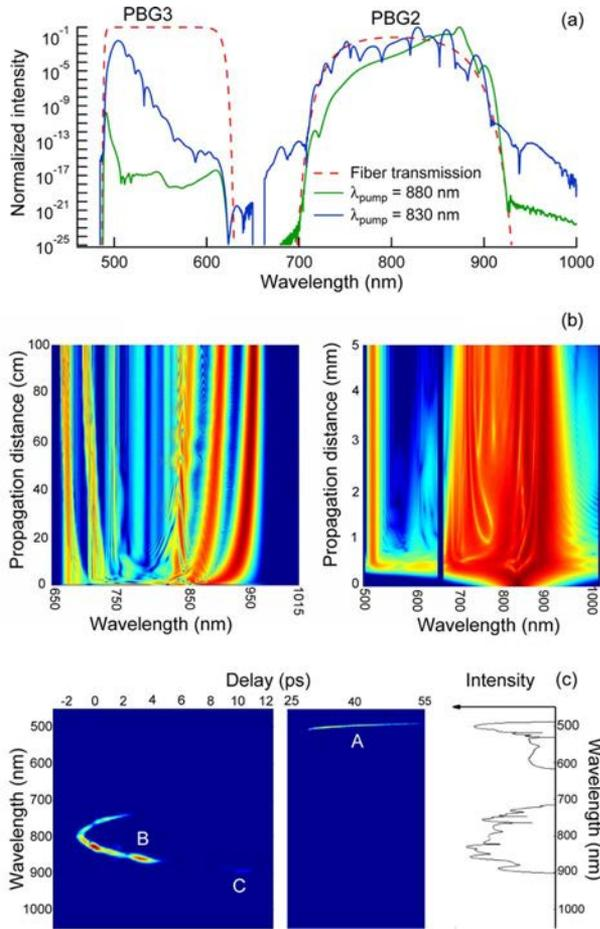
Fig. 3. (Color online) (a) Output spectra after 50 cm propagation for pump wavelengths as shown. (b) SC evolution in PBG2 over fiber length of 1 m with  $\alpha = 0$  (left) and simulated SC evolution in PBG2 and PBG3 over a propagation distance of 5 mm ( $\lambda_{\text{pump}} = 830 \text{ nm}$ ,  $P_{\text{in}} = 100 \text{ kW}$ ) (right). (c) Output spectrogram correlating DW (A) and solitons (B) and (C).
