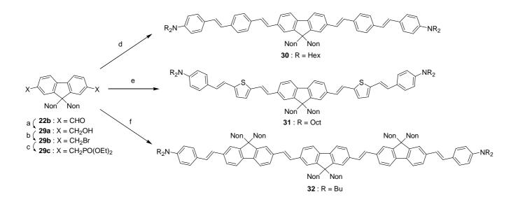
**Scheme 7.** Reagents and conditions: (a) KBH<sub>4</sub>, EtOH/CH<sub>2</sub>Cl<sub>2</sub>, 20 °C, 14 h (97%); (b) concd HBr, reflux, 3 h (90%); (c) P(OEt)<sub>3</sub>, reflux, 60 h (62%); (d) **4b** (2.2 equiv), NaH, THF, 20 °C, 20 h (53%); (e) **6b** (2.5 equiv), NaH, THF, 18-crown-6 cat, reflux, 7 h (68%); (f) **25** (2.2 equiv), NaH, THF, 20 °C, 16 h (84%).
