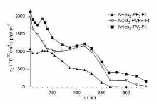
Figure 12. TPA spectra in toluene of 19b, 20 and 30: linker effect.
