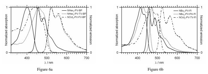
Figure 6. Absorption and emission spectra in toluene of (a) 16a, 17b and 17a; (b) 24, 32 and 31: length effects.
