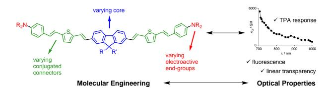
A comprehensive series of push-push and pull-pull fluorophores was prepared from the symmetrical functionalization of an ambivalent core with conjugated rods bearing acceptor or donor end-groups. Their absorption, photoluminescence and two-photon absorption (TPA) properties have been investigated, allowing to derive structure-property relationships and to lay guidelines for both spectral tuning and amplification of TPA.
