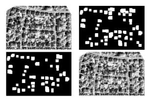
Fig. 3. Input image (top left), filtered image (top right), detected objects (bottom left), and final result (bottom right) on one of the test images.
