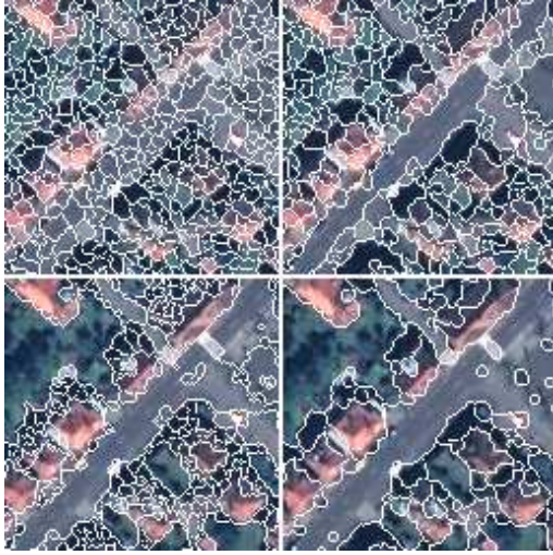
Fig. 6. Visual comparative results: unsupervised watershed (top left), evolutionary unsupervised watershed (top right), supervised watershed (bottom left), and evolutionary supervised watershed (bottom right).
