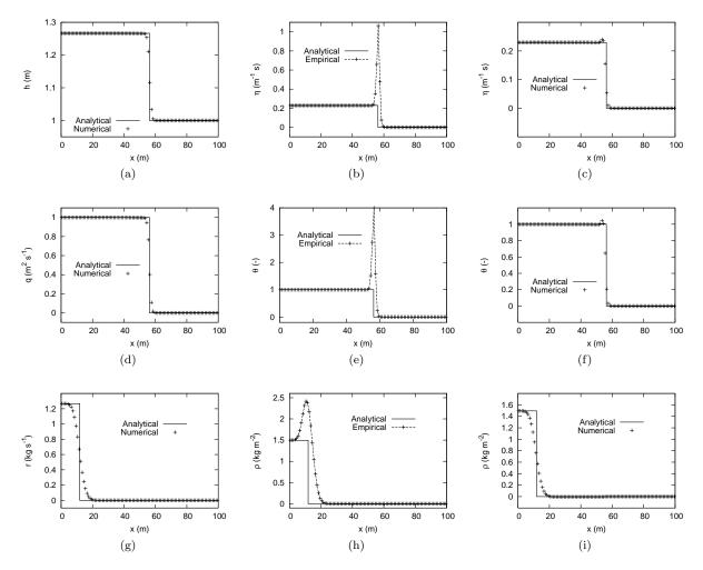
Figure 6: Bore propagation into a frictionless channel and sensitivity with respect to the prescribed unit discharge  $q_b$ . Left: flow solution, middle: empirical sensitivity, right: numerical sensitivity.
