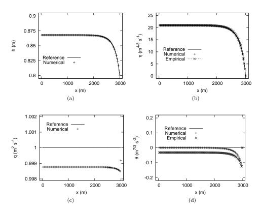
Figure 1: Sensitivity to the Manning coefficient for a steady state flow on a sloping bed. Comparison between the proposed solver and the explicit Euler method (reference). For the sake of clarity, only one point every 25 is represented.
