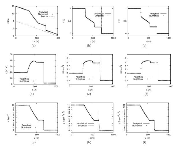
Figure 4: Dam-break problem on a positive slope. Left: flow solution, middle: empirical sensitivity, right: numerical sensitivity. For the sake of clarity, only one point every 100 is represented. The values reached by the peaks in subfigures (b) and (e) are respectively about 175 and 2130.
