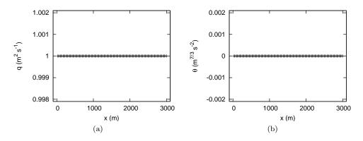
Figure 2: Sensitivity to the Manning coefficient for a steady state flow on a sloping bed. Values of q and  $\theta$  computed at the interfaces.
