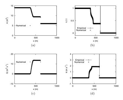
Figure 7: Dambreak problem for a trapezoidal channel. Left: flow solution, right: empirical and numerical sensitivities.
