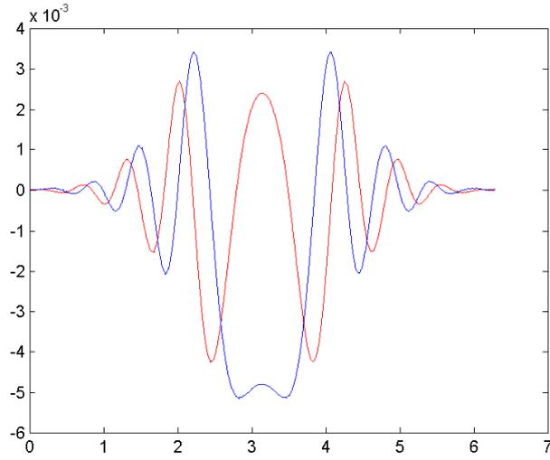
(b) The real (in red) and imaginary (in blue) parts of the current  $\mathbf{j}$ , in  $A/m$ , of the virtual antenna, in function of the polar angle.
