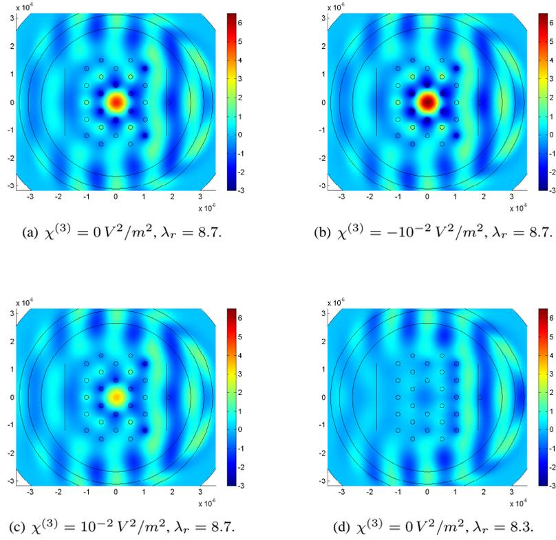
Figure 3: The real part of the total electric field  $\Re e\{u\}$ , in  $V/m$ , for different values of  $\chi^{(3)}$  (zero in 3(a) and 3(d), negative in 3(b) and positive in 3(c)) and different wavelengths (the resonant wavelength  $\lambda_r = \lambda_a$  in 3(a), 3(b) and 3(c), and in the gap in 3(d)).
