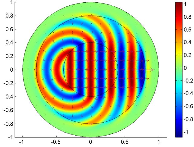
(a) The real part  $\Re\{u_v^i\}$ , in  $V/m$ , of the field generated by the virtual antenna, and arrows of the line density of the average over a time period of the electromagnetic power  $\mathcal{P}_e^{harm}$ , in  $W/m^2$ .
