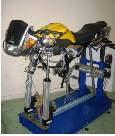
Fig. 1. The developed riding motorcycle simulator by INRETS-UEVE-UPSUD
