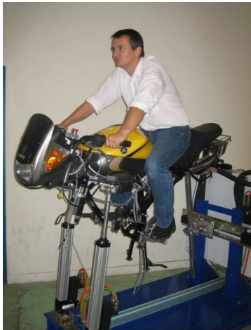
Fig. 15. Constructed riding motorcycle simulator
