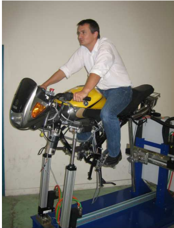
Fig. 15. Constructed riding motorcycle simulator
