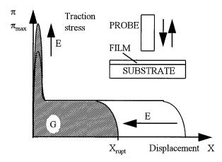
FIG. 1. Typical stress curve observed (Ref. [7]) at imposed displacement (constant separation rate). The traction force increases sharply upon separation. It then strongly decreases again and reaches a plateau, until it decreases further to zero. Our model predicts that the plateau should shorten and that the peak should increase with increasing modulus E (see Fig. 5). Inset: Usual experimental geometry.
