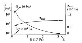
FIG. 5. Predictions of the model, using the parameter values given in the text, and taking  $\tau_{\rm f}={\rm const.}$  The tack energy G has a strong dependence on the elastic modulus E, whereas the traction peak  $\pi_{\rm max}$  varies mildly.
