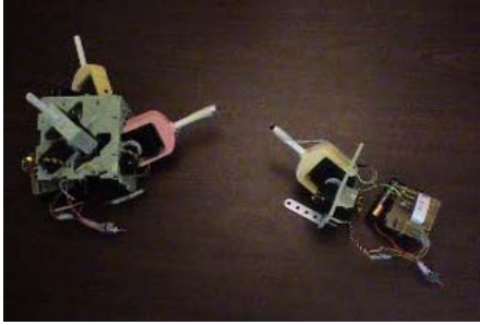
Fig. 15. Communication between two robots. The left robot commands the other with remote invocations, during the alignment of legs.
