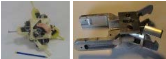
Fig. 4. Prototypes of the maam robot. They embed all the electronic and software described in this paper, but do not include the pincers.
