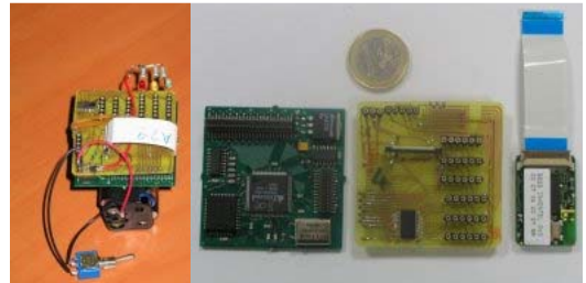
Fig. 6. Embedded electronic: CPU, extension card and industrial bluetooth module.
