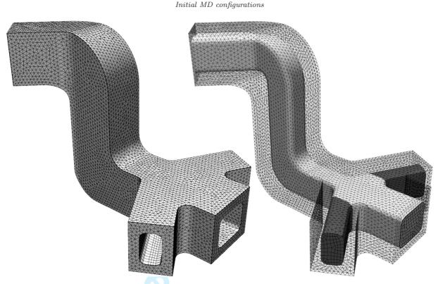
Figure 1. A complex geometry test case: a three-inlet fluid mixing channel. Four zones are defined, the exterior region (left) contains a tethered crystal lattice to define the channel walls. The three interior zones (right, one central and two 'arm' zones) contain the molecules representing the liquid. The overall height of the system is 82nm.
