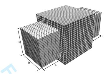
Figure 16. Two examples of the mesh used for examining aspect ratio sensitivity: a = 1 (dark, white grid) and  $a = (40/28)^3 = 2.915$  (light, black grid). Note that the number of cells is the same in both cases (20 in each direction); they are stretched to match the overall dimensions.
