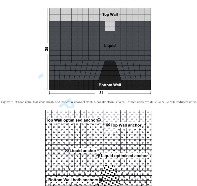
Figure 8. Three zone test case configuration of molecules. Molecules coloured according to id. User specified anchors 🛞 and optimised anchors  $\bigoplus$  are shown.
