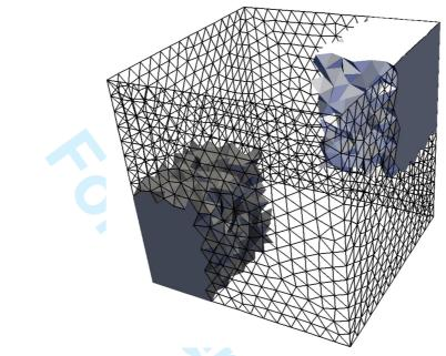
Figure 13. Tetrahedral test mesh with edge number 15. The outline of cells on four of the six faces of the bounding cube are shown, and two of the twelve portions of cells are shown from the mesh when decomposed for parallelisation.
