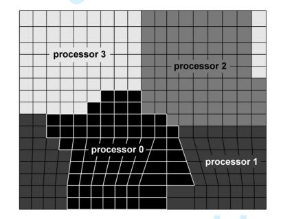
Figure 10. The mesh for the three zone test case decomposed into 4 portions for parallelisation. Processors 1 and 3 have zones with disconnected volumes.
