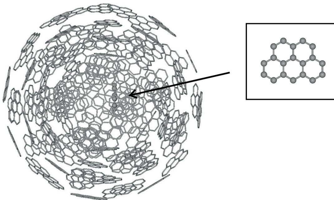
FIG. 1: Geometry of the soot particle used in the GCMC calculations. It is made of 113 small  $C_{19}$  units of 19 carbon atoms randomly arranged on the surface of four concentric spheres (see text) and one additional  $C_{19}$  unit located in the middle of the system. The  $C_{19}$  unit is shown in the inset.
