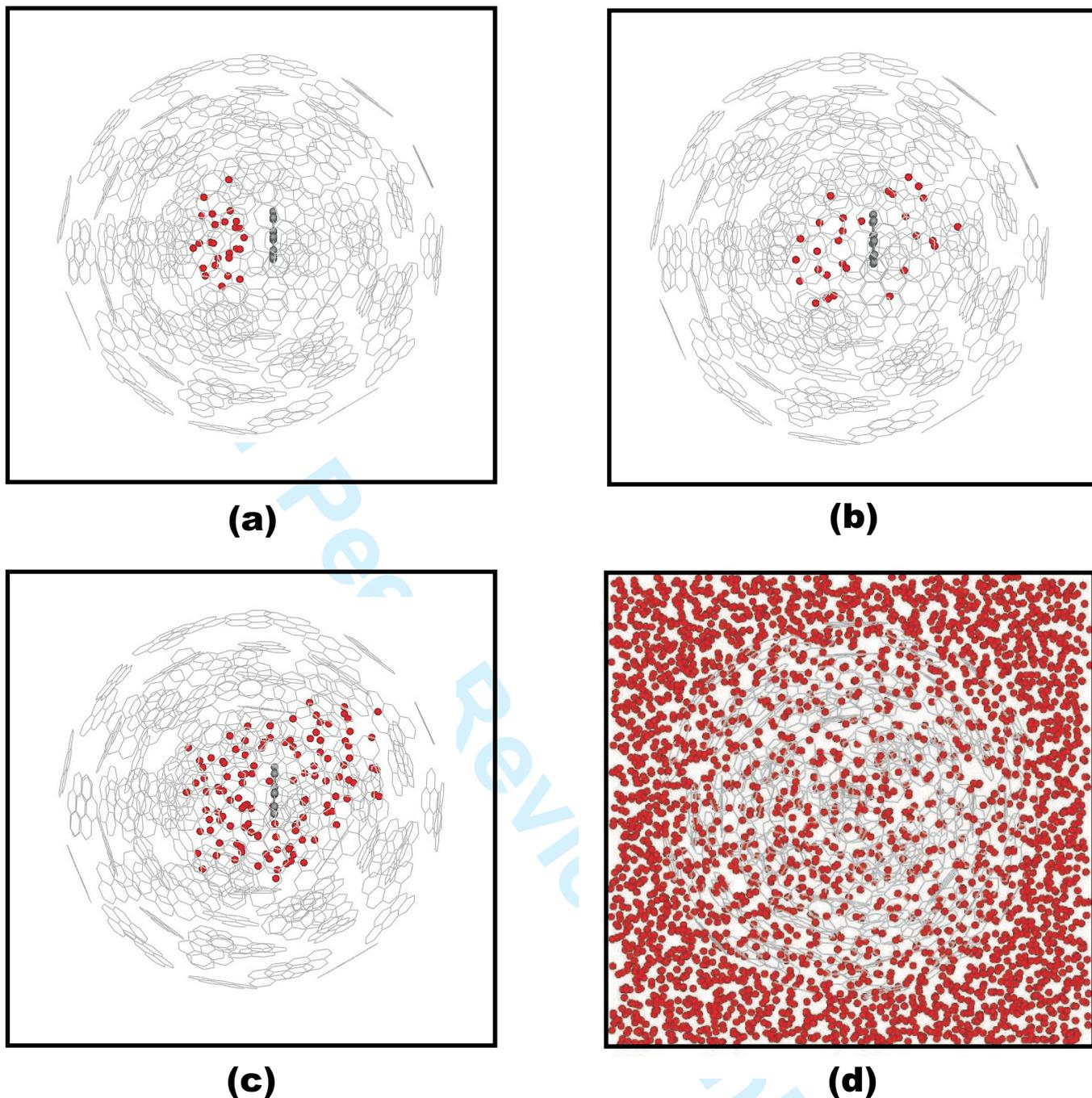
FIG. 3: Configurations of water molecules adsorbed at 298 K on the soot particle corresponding to different parts of the isotherm. The oxygen atoms of water are represented as circles, and the hydrogen atoms have been masked for clarity. The carbon atoms of the  $C_{19}$  unit located inside the soot particle are also represented as grey circles.
