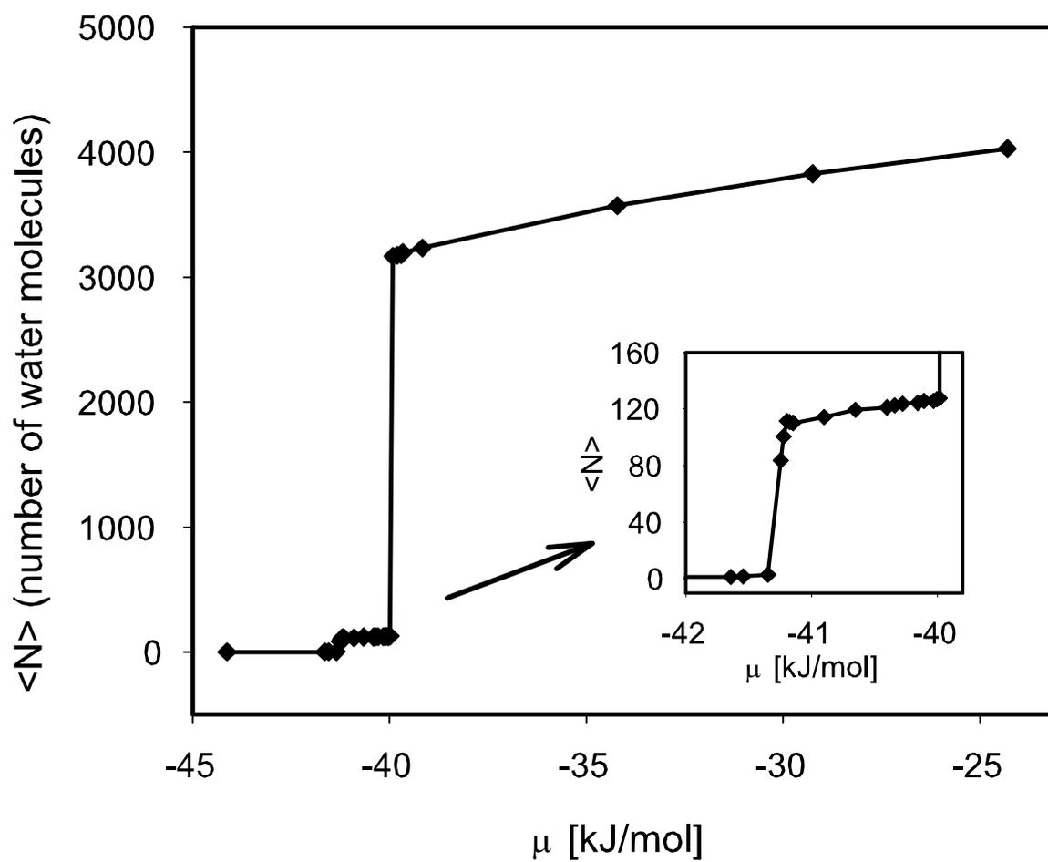
FIG. 2: Water adsorption isotherm on the soot particle as a function of the water chemical potential at 298 K. The inset shows the region of the first plateau on a magnified scale.
