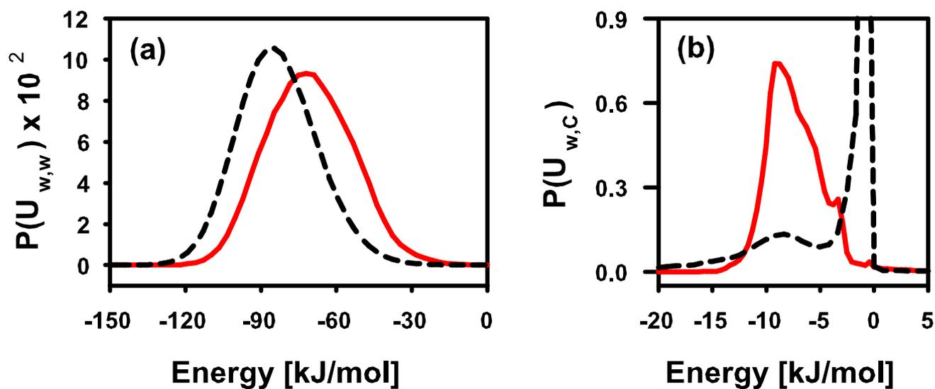
FIG. 4: Distribution of the energy of (a) water-water ( $U_{w,w}$ ) and (b) water-carbon ( $U_{w,C}$ ) interaction of a single water molecule for two typical values of the water chemical potential, i.e.,  $\mu = -40.90$  kJ/mol (full curves) and  $\mu = -39.81$  kJ/mol (dashed curves). Note that the main peak in the distribution of water-carbon energy for  $\mu = -39.81$  kJ/mol has been cut off since it corresponds to liquid water molecules having negligible interaction with the soot particle.
