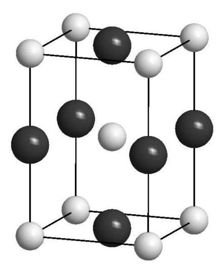
Figure 8. Average tetragonal crystal structure of the high-pressure modification of Cu<sub>3</sub>N from experimental data. White spheres correspond to copper atoms. Nitrogen positions (dark spheres) are only occupied to  $1/3^{rd}$ . 162x178mm (96 x 96 DPI)
