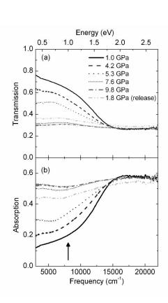
Figure 9. (a) Transmission  $T(\omega) = I_s(\omega)/I_r(\omega)$  (see text for definitions) of Cu<sub>3</sub>N at ambient temperature as a function of pressure and (b) the corresponding absorption  $_A = \log_{10}(1/T)$  as a function of pressure. The arrow in (b) indicates the frequency position of the absorption edge. 558x431mm (150 x 150 DPI)
