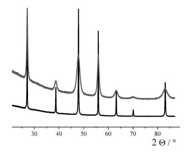
Figure 2. XRD pattern of LP-Cu<sub>3</sub>N before (bottom line) and after (top line) a pressure treatment in the multi-anvil cell at about 9 GPA (Co-Ka1 radiation). 594x419mm (150 x 150 DPI)
