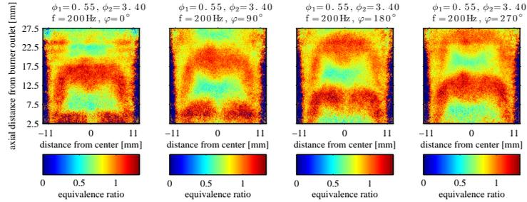
Figure 11: Equivalence ratio distributions in nonreactive conditions for four phase angles  $\varphi$ . The excitation frequency is  $f = 200$  Hz, the equivalence ratios of the primary and the injected flow are  $\phi_1 = 3.40$  and  $\phi_2 = 0.55$  respectively and the blowing ratio is  $\overline{BR} = 3$ . Propane is used in this experiment used to augment the signal to noise ratio.
