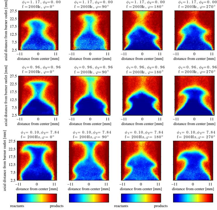
Figure 12: Mean flame front for a modulation at 200 Hz and an average equivalence ratio  $\phi = 0.96$ . Top row :  $\phi_1 = 1.17, \phi_2 = 0.00$ . Middle row :  $\phi_1 = 0.96, \phi_2 = 0.96$ . Bottom row :  $\phi_1 = 0.10, \phi_2 = 7.84$ .
