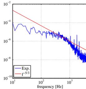
Figure 10: Power spectral density (PSD) of the velocity signal measured in the duct exhaust section obtained using hot-wire anemometry. Secondary injection is switched on with  $BR = 3$ . The red graph represents the  $f^{-5/3}$  spectral decay.
