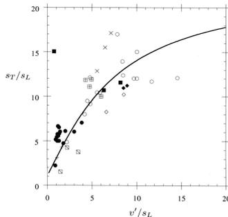
Figure 16: Turbulent flame speed as a function of the turbulence intensity  $v'$ . Experimental results correspond to Reynolds numbers ranging from  $Re_t = 500$  - 750 and the calculated burning velocity model is for  $Re_t = 625$  (originating from Peters (2000))
