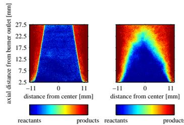
Figure 8: Mean flame front of the laminar flame on the left and the turbulent flame on the right. Conditions are  $\phi = 0.96$  in both cases and the turbulent flame is subject to an injection flow with  $BR = 3$ .
