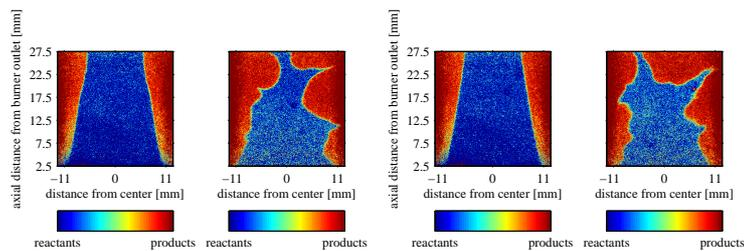
Figure 9: **Typical** single shots of the flame front. The laminar flame is on the left and the injection-induced turbulent flame on the right. Same conditions as in Fig. 8.
