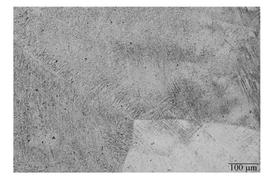
Optical micrographs show  $\beta$ -prior grains (a),  $\beta$ -prior grains and  $\alpha$ -plates within them (b) and mainly  $\alpha$ -phase (c) in the alloys 131, 129 and 134, respectively. 83x56mm (300 x 300 DPI)
