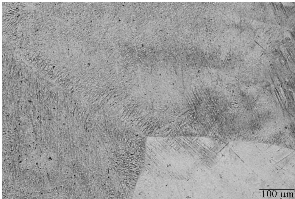
Optical micrographs show  $\beta$ -prior grains (a),  $\beta$ -prior grains and  $\alpha$ -plates within them (b) and mainly  $\alpha$ -phase (c) in the alloys 131, 129 and 134, respectively.
