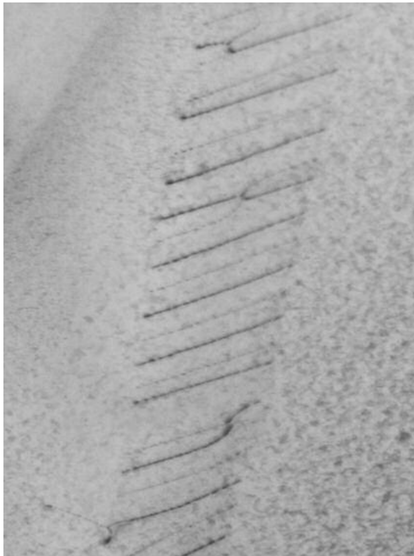
Figure 1b: Zoom-in on region A showing the detailed structure of the wall with successive dislocations exhibiting different contrasts.
