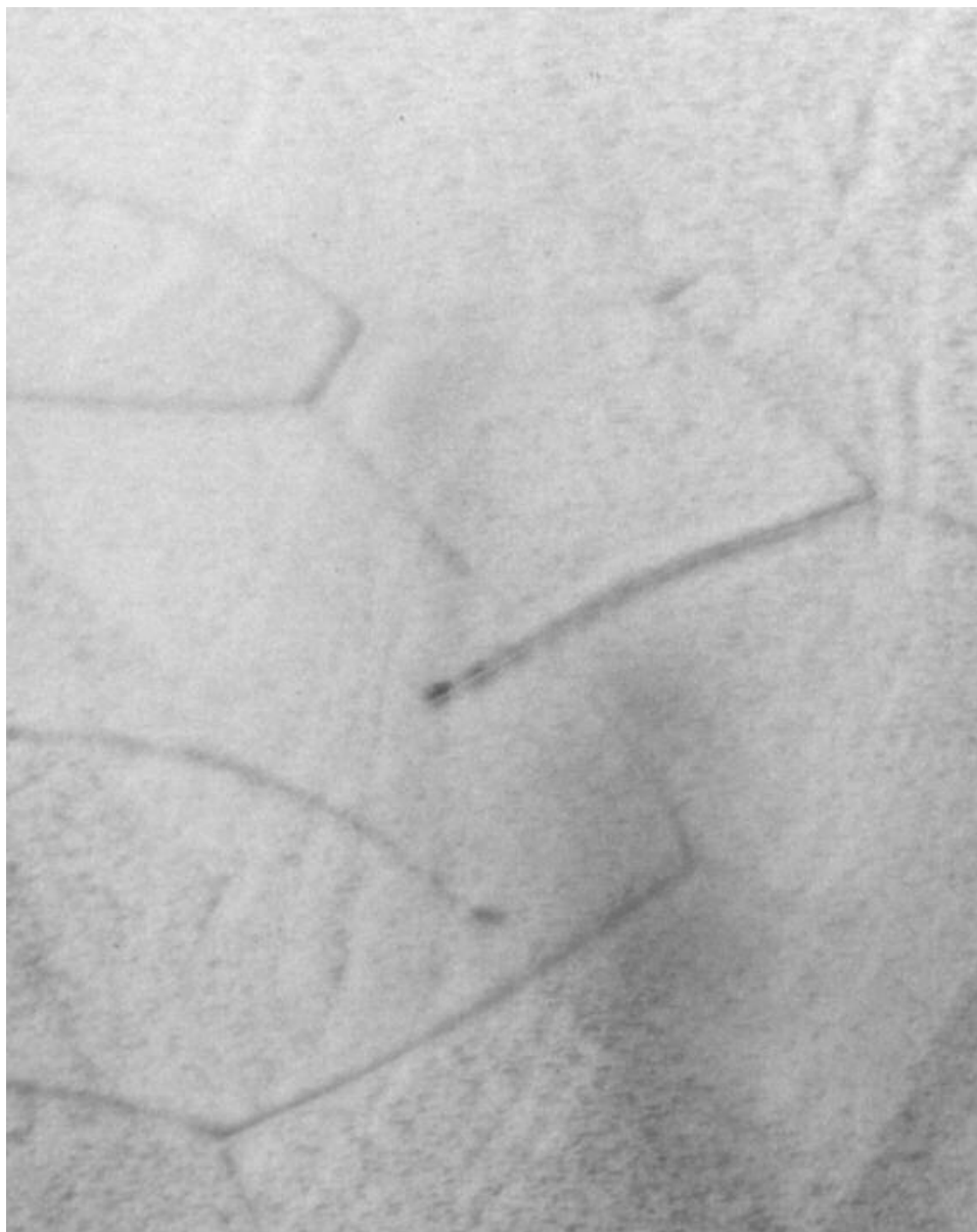
Figure 1c: Zoom-in on region B revealing dislocation network with out-of-basal-plane segments.
