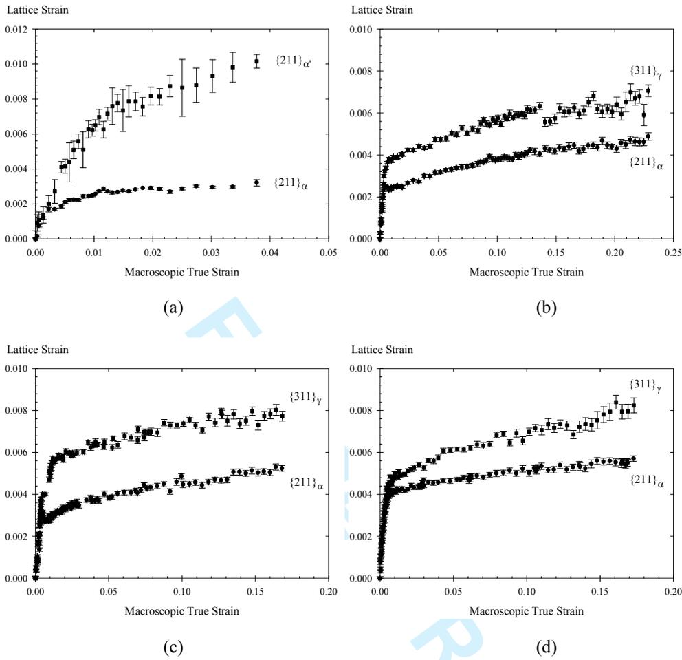
Figure 7: Evolution of the BCC, BCT or FCC lattice strains in the loading direction as a function of the macroscopic strain for specimens DP (a), TRIP1 (b), TRIP2 (c) and B (d).
