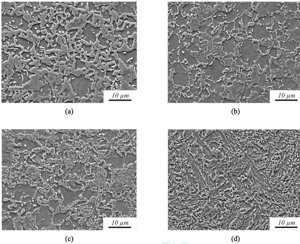
Figure 1: SEM micrographs of the 4 microstructures considered in this study. They correspond to specimens DP (a), TRIP1 (b), TRIP2 (c) and B (d).
