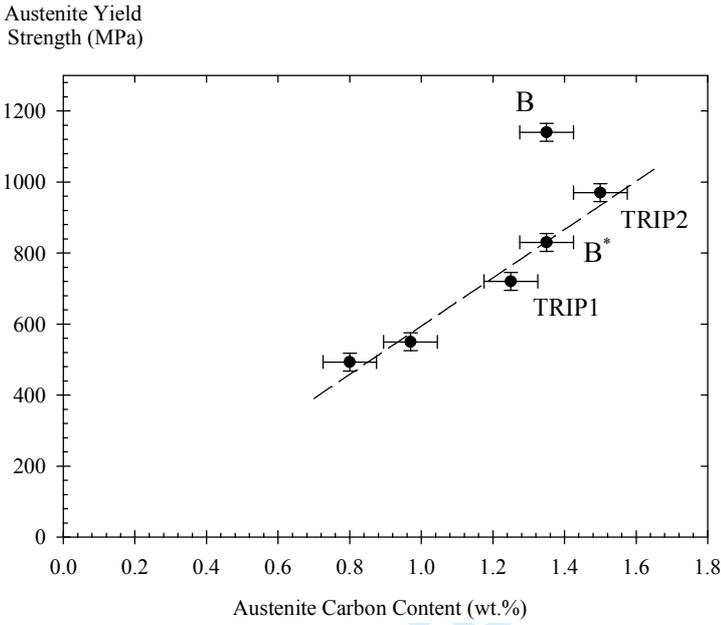
Figure 14: Evolution of the austenite yield strength as a function of its carbon content for several TRIP-assisted multiphase steels.
