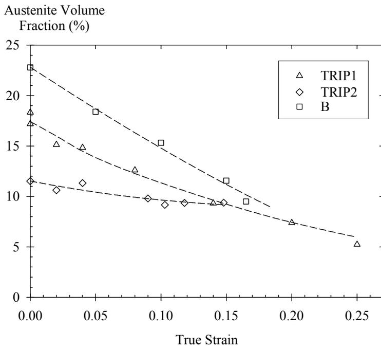
Figure 3 : Austenite transformation rate during uniaxial tension for specimens B, TRIP1 and TRIP2.
