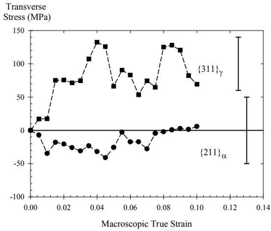
Figure 10: Transverse stresses in BCC and FCC lattices calculated using equation (2b) as a function of the macroscopic true strain for specimen TRIP2.
