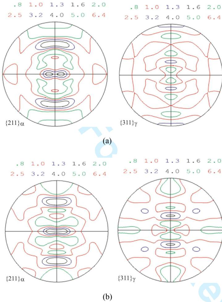
Figure 4 :  $\{211\}_\alpha$  and  $\{311\}_\gamma$  pole figures of specimen TRIP1 before any straining (a) and at the onset of necking (b).
