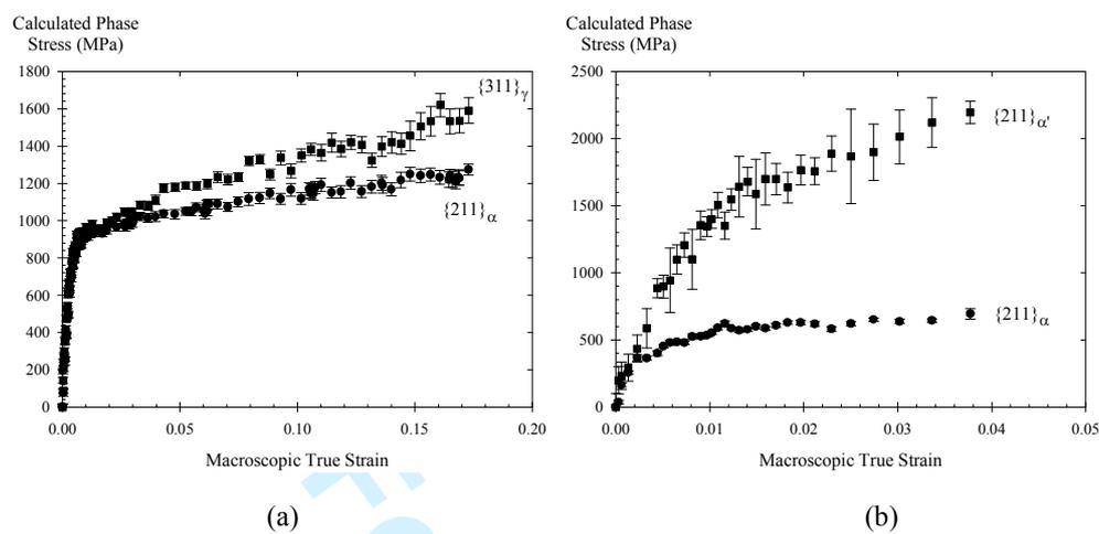
Figure 11: Evolution of the FCC and BCC or BCC and BCT phases as a function of the macroscopic true strain for specimens B (a) and DP (b).
