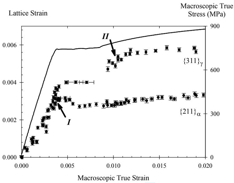
Figure 13: Comparison of the evolutions with true strain of the true stress and the BCC and FCC lattice strains in the case of specimen TRIP2.
