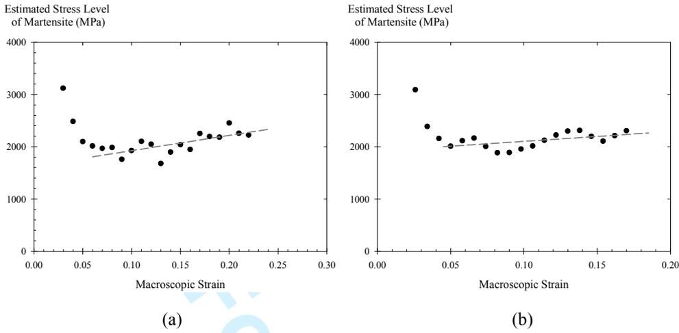
Figure 17: Estimated stress level of the martensite during straining of specimens TRIP1 (a) and B (b).
