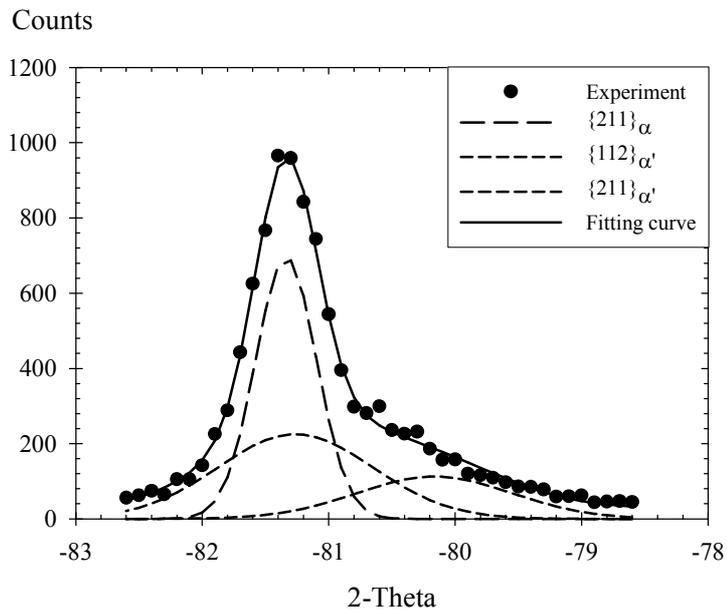
Figure 6 : Peak shape resulting from the superposition of the  $\{211\}_\alpha$ ,  $\{211\}_{\alpha'}$  and  $\{112\}_{\alpha'}$  peaks in specimen DP and dotted curves corresponding to the deconvoluted peaks.
