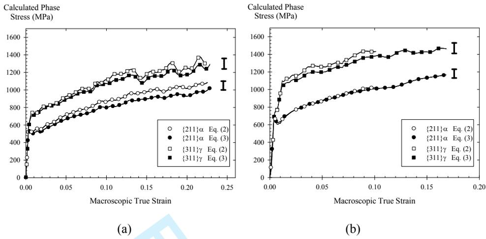
Figure 9: Comparison of the longitudinal stresses in BCC and FCC lattices calculated using equations (2a) or (3) as a function of the macroscopic true strain for specimens TRIP1 (a) and TRIP2 (b).
