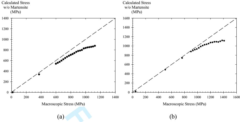
Figure 16: Comparison of the macroscopic true stress and the stress recalculated from the lattice strains by the mechanical equilibrium for specimens TRIP1 (a) and B (b).
