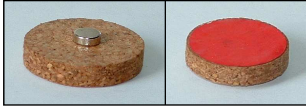
FIG. 1: (Color online) Magnetized particle attached to a cork disc of larger diameter ( left ). The composite particle can float upside down on the surface of water ( right ). The diameter d and height h values are d = 4 mm and h = 1.5 mm, and d = 26 mm and h = 5 mm, for the magnetic particle and cork disc, respectively.
