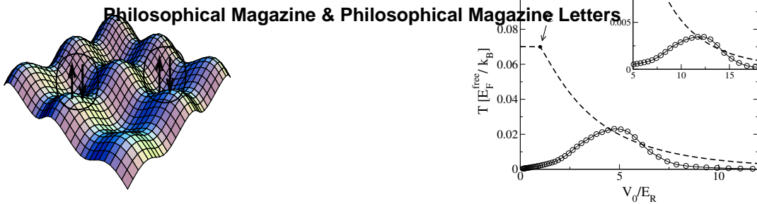
FIG. 2: Left: Fermions with attractive interaction forming Cooper pairs in an optical lattice. Right: Critical temperature for the SF transition of \text{Li}^6 atoms as a function of the optical lattice depth in a 3d \text{CO}_2 lattice. Inset: analogous plot for \text{K}^{40} atoms in a Nd:YAG lattice. The dashed curves show the effect of adiabatic cooling if the atoms are loaded into a weak lattice at point C which is then decoupled from the reservoir. Figures taken from (Hofstetter et al. 2002).
