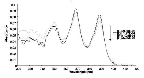
**Figure 4.** The changes in the absorption spectra of **3a** upon titration with F<sup>-</sup> upon excitation of 369 nm, in DMSO.
