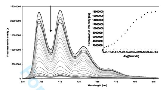
**Figure 6.** Fluorescence titration spectra showing the changes in fluorescence emission of **3a** in DMSO upon addition of fluoride, from top to bottom,  $[F^-]=0 \rightarrow 1.1 \times 10^{-1}$  M. Insert: The changes in the 415 nm transition as a function of  $[F^-]$ .
