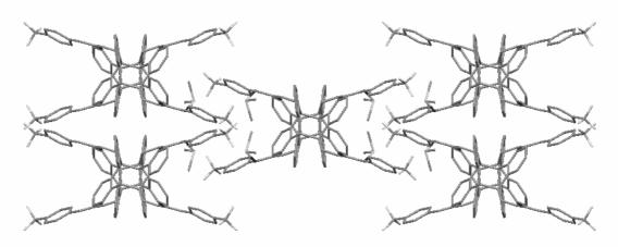
**Figure 2**. The packing diagram for **4** by viewing down the c-axis. Hydrogen atoms and short-contacts have been removed for clarity.
