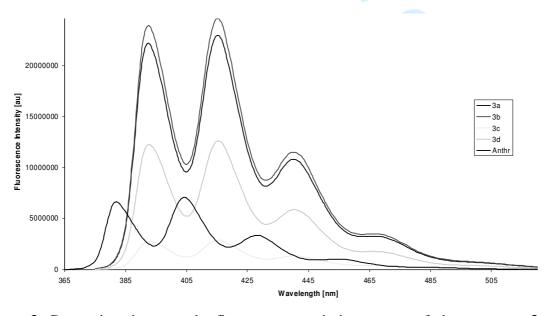
**Figure 3.** Comparison between the fluorescence emission spectra of chemosensors **3a-d** and the spectrum of anthracene, **Anthr**, in DMSO.
