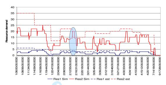
Figure 7. Simulation results, obtained for the packaging section of the plant (1-week period). Considered disturbances are simulated machine breakdowns (day 2, 3x2hours) and stochastic processing times.
