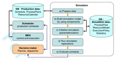
Figure 6. Architecture and the main process flow in the simulation module.
