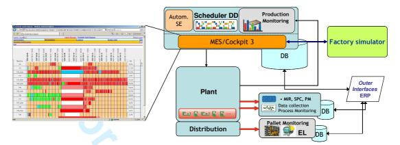
Figure 4. Structure of the realized system and the graphical user interface (GUI) of the MES Cockpit.
