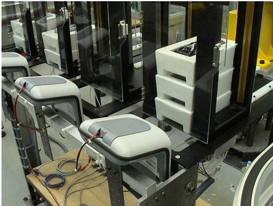
Figure 8: Work in process buffer for packing robot.
