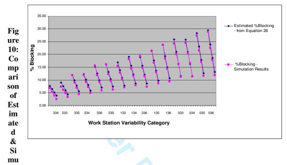
lated %Blocking on 5 Workstation Flow Lines: Zero Blocking on 5<sup>th</sup> Workstation
