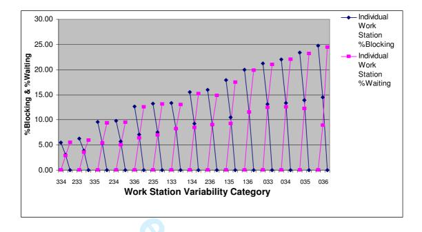
Figure 5: % Blocking and % Waiting on 3 Workstation Flow Lines
