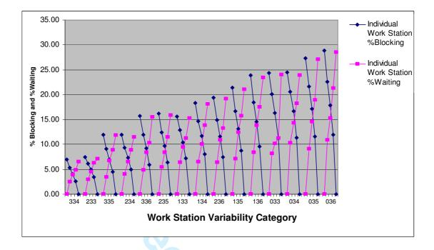
Figure 6: % Blocking and % Waiting on 5 Workstation Flow Lines
