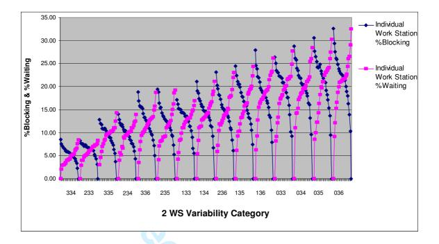
Figure 9: % Blocking and % Waiting on 21 Workstation Flow Lines
