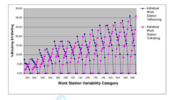
Figure 7: % Blocking and % Waiting on 8 Workstation Flow Lines
