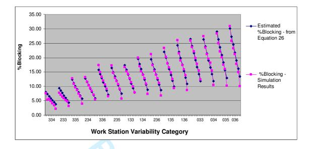
Figure 11: Comparison of Estimated & Simulated % Blocking on 8 Workstation Flow Lines: : Zero Blocking on 8<sup>th</sup> Workstation
