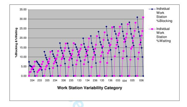
Figure 8: % Blocking and % Waiting on 13 Workstation Flow Lines
