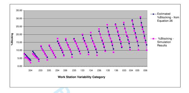
Figure 12: Comparison of Estimated & Simulated % Blocking on 3 Workstation Flow Lines : Zero Blocking on 13<sup>th</sup> Workstation
