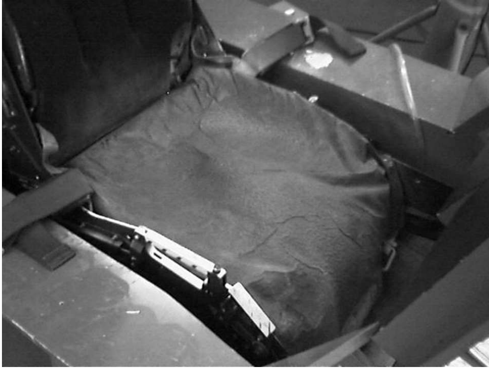
Figure 2. Photograph of Burnett Seat in position, shown with a custom seat profile 254x190mm (96 x 96 DPI)
