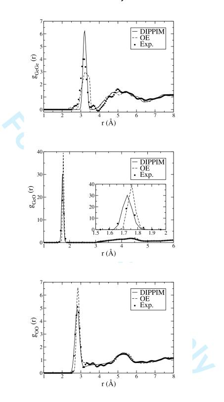
FIG. 2: Radial distribution functions obtained from the 300 K simulations with the DIPPIM and original OE interaction potentials. These are compared to the experimental ones obtained from neutron diffraction experiments<sup>5</sup>.
