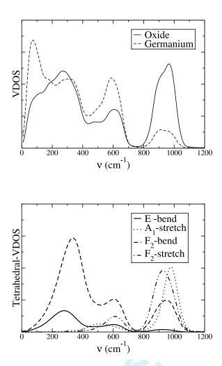
FIG. 7: The vibrational densities of states, for the DIPPIM, of both type of ions (top panel), and their projections in terms of the A (symmetric stretch),  $F_2$  (asymmetric stretch), E (bend), and  $F_2$  (bend) modes of the GeO<sub>4</sub> tetrahedra (bottom panel).
