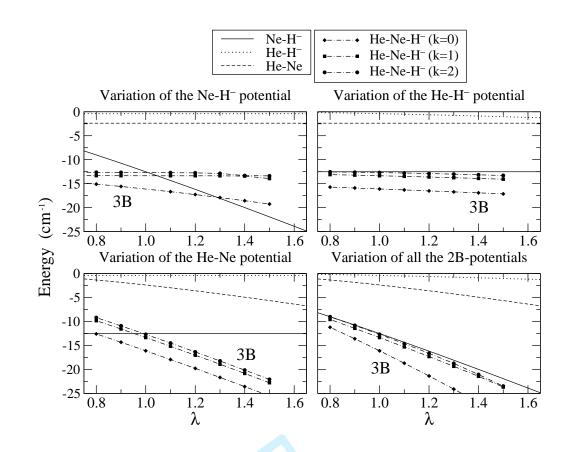
FIG. 12: Same as in figure 11 but for the anionic system. Three of the panels show the effect on the 3B energy as each of the 2B potentials is varied, while the fourth panel (bottom right) shows 3B energy variation as all the three 2B potentials are varied.
