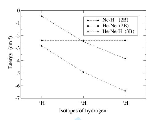
FIG. 9: Sequential presentation of the energy thresholds in the HeNeH complex as a function of the three isotopic variants containing <sup>1</sup>H (left panel), D (central panel) or T (right panel).
