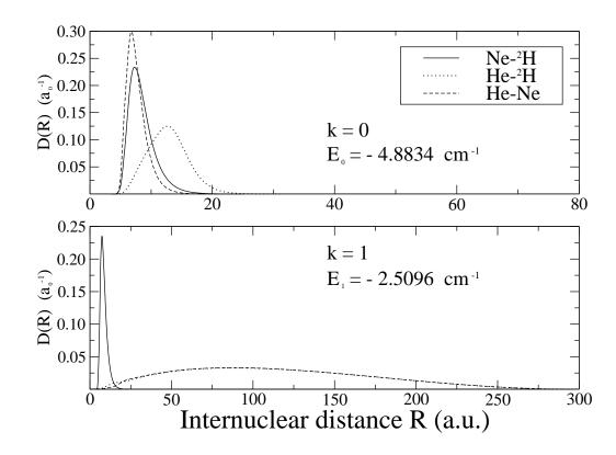
FIG. 8: Atom-atom radial density distributions  $(a_0^{-1})$  computed in the deuterated complex Ne<sup>2</sup>HHe. The symbols are explained within the figure.
