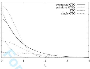
Figure 2. Radial behaviour of the 1s-contracted GTO of the hydrogen atom in the STO-3G basis set [107], the three primitive GTOs that form it, the STO that is meant to be approximated and a single GTO with the same norm and exponent as the STO. The notation  $r_a$  is shorthand for the distance to the  $\alpha_a$ -th nucleus  $|\boldsymbol{r} - \boldsymbol{R}_{\alpha_a}|$ .
