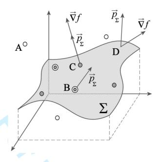
Figure B1. Schematic depiction of a constrained stationary points problem.  $\Sigma$  is the 2-dimensional search space, which is embedded in  $\mathbb{R}^3$ . The white-filled circles are solutions of the unconstrained problem only, the gray-filled circles are solutions of only the constrained one and the gray-filled circles inside white-filled circles are solutions of both. A, B, C and D are examples of different situations discussed in the text.
