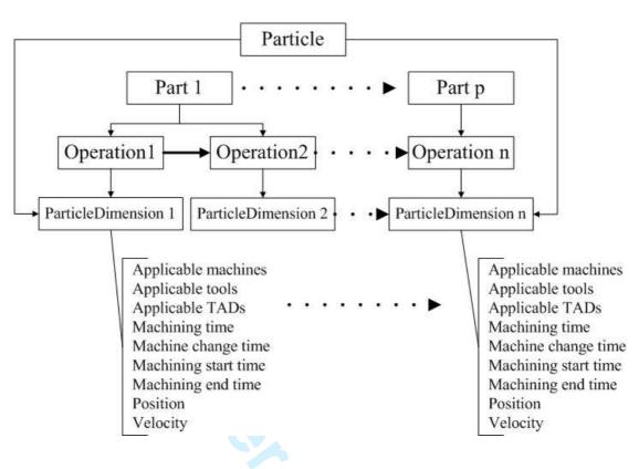
Figure 2 Representation of a solution for IPPS problem
