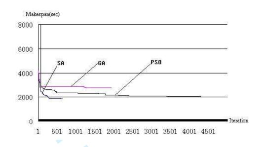
Figure 8 Comparison of GA, SA and PSO of Makespan for Group 1 (8 mins' run)
