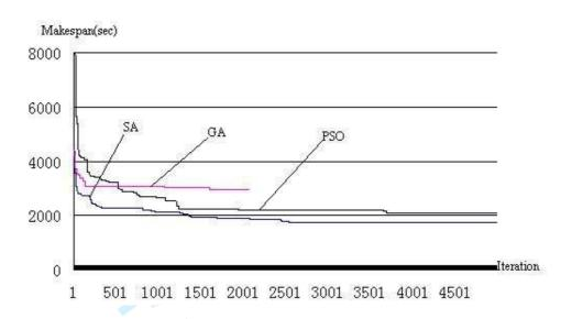
Figure 12 Comparison of PSO, GA and SA of Makespan for Group 2 (in 7 min)
