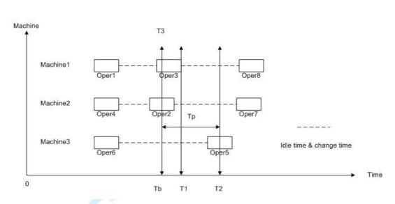
Figure 3 Determination of machines available times when machine2 breaks down
