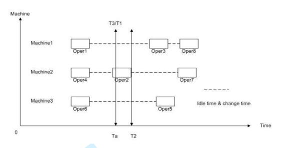
Figure 4 Determination of available times for machines when new order arrives at T<sub>a</sub>
