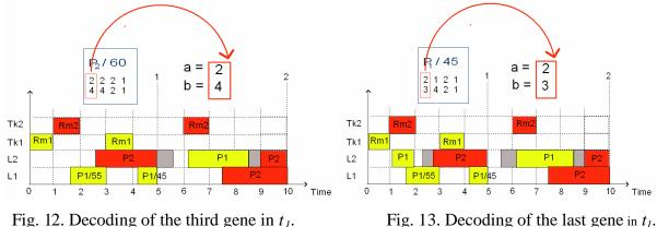
The final schedule established by the decoding procedure for lines and tanks is a possible solution for the problem which is evaluated using the fitness function. The objective function of the mathematical formulation described in Toledo (2005) and Toledo *et al.* (2006) is the fitness function in the GA. To sum up, this value is determined adding up all costs that happen in the final schedule: setup, production
