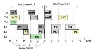
Fig. 2. Synchronization between lines and tank slots
