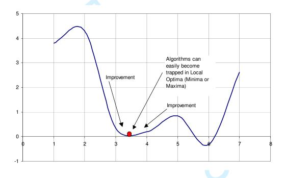
Figure 1 – Trapping at Local Optima (minimising algorithm).
