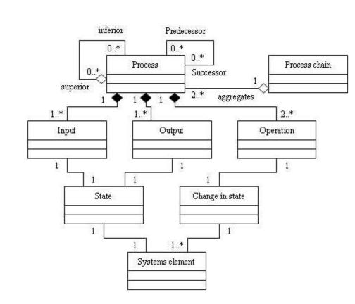
Figure 1: Class diagram of a general process chain 77x63mm (150 x 150 DPI)
